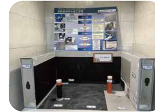
Waterproofing construction method demonstration
